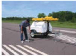
1. Level as necessary using 3 leveling jacks
