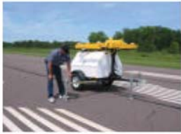
1. Level as necessary using 3 leveling jacks
