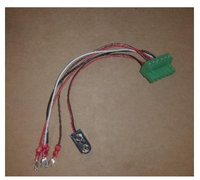
3) At the (2) terminal blocks, one-by-one remove each wire that leads to old tilt switch and replace with same color wire from new harness.
