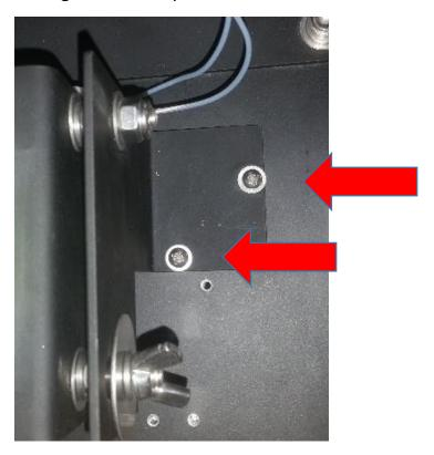
5) Use the same hardware and same mounting holes to install the Retrofit Kit.
