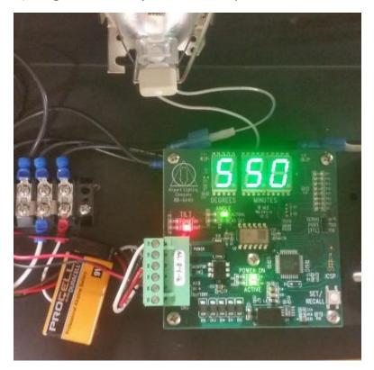
7) Begin rotating the angle adjustment screw to bring the sensor as close to a level position "0 00" as possible. (+/- 0 05 is acceptable).
