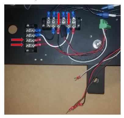
4) Remove (2) screws, washers and lock washers that mount the old Tilt Switch to the Light Unit baseplate.
