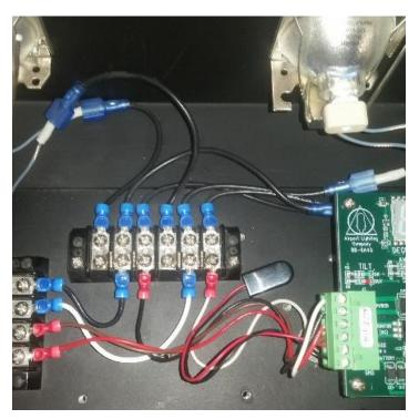
7) Plug a 9V battery into the adapter on the harness. The board will power on.
