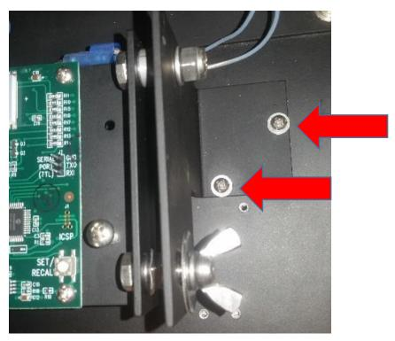
6) Plug the harness back into the circuit board. Loosen the wingnut on the right side of the Retrofit Kit until the bracket swivels freely.
