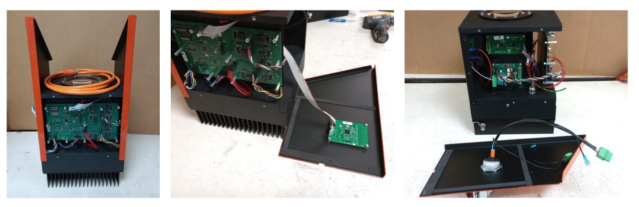
Unplug the Power Supply Tray from the 88-00400 PCBRemove the Power Supply Tray
