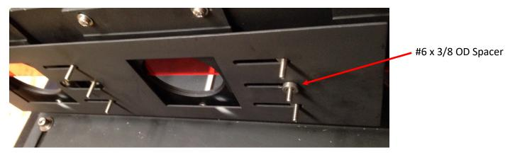
6) Install exterior baffle so that the large hole on baffle fits around the #6 x 3/8 OD spacer.
