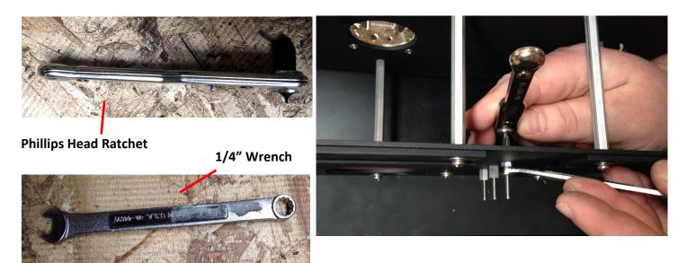
3) Add (1) #6 Washer part # 99-00090 to all screws except the center, left screw (pointed out below).
