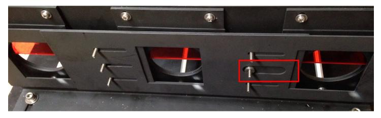
7) Install (1) #6 washer part # **99-00090** on all screws except the one that already has a #6 x 3/8 OD spacer. Next, add (1) #6 lock washer part # **99-00088** and (1) 6-32 hex nut part # **99-00061** to all six screws. DO NOT TIGHTEN HARDWARE YET.
