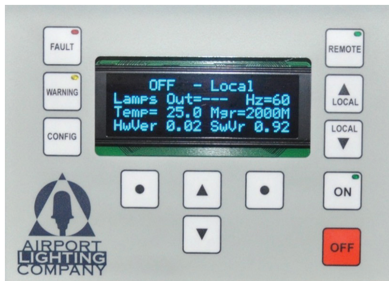
Figure 14: Megger Measurement (Open Circuit)
