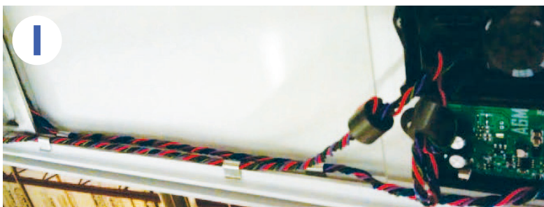
C7-LVCV2 power supply and C7-DRVR driver with wire harnesses secured by u-clips.
