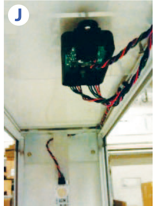
Additional C7-DRVR driver mounted in the sign top. Wire harnesses secured with wire u-clips to prevent sagging.
