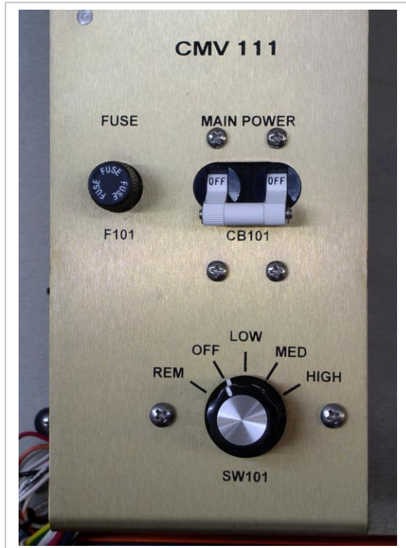
Figure 11a CMV-111 Control Module
