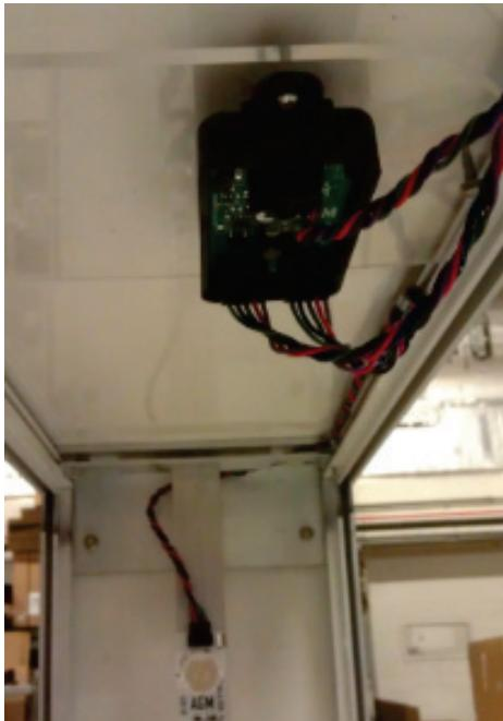
[j] Additional C7-DRV driver mounted in the sign top. Wire harnesses secured with wire u-clips to prevent sagging.
