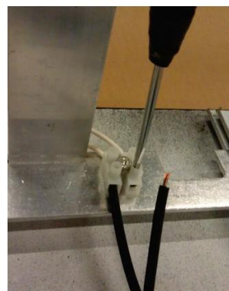
Do not tighten the hex head screws so far as to cause the mounting bracket to bend (the head of the screw does not need to touch the metal to secure the bracket).
