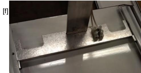
12. Insert mounting bracket #1. Slide the mounting bracket in the mounting channels, with the LEDs facing into the sign, until it contacts the u-clips used as stops [f].
