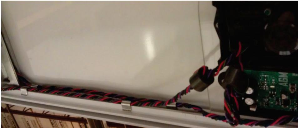
[i] C7-LVCV2 power supply and C7-DRV driver with wire harnesses secured by u-clips.
