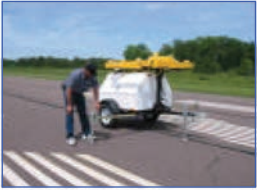
1. Level as necessary using 4 leveling jacks
