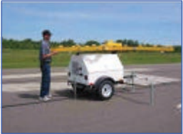
2. Extend the 4 light assembly arms
