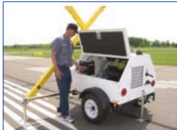
4. Start the generator and activate the lights
