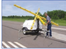
3. Tilt the light to the upright position
