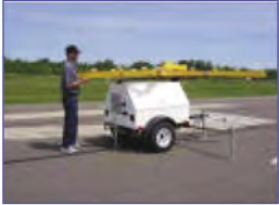
2. Extend the 4 light assembly arms
