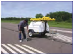
1. Level as necessary using 4 leveling jacks
