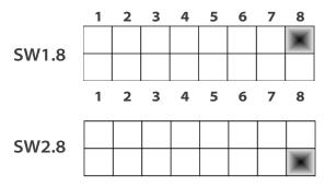
**Test Mode 2:** Used when calibrating new LED boards. Unit ignores RS485 Comm faults. LHA ID must be set to LHA1.
