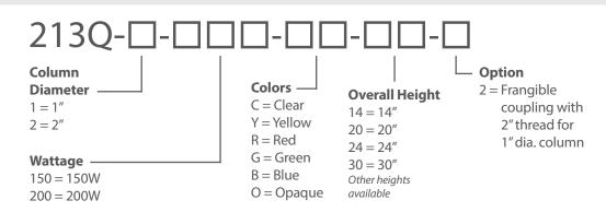
Example: 213Q-1-200-RG-24 is a 213Q fixture with 1" column, 200W lamp, red/green and 24" overall height
