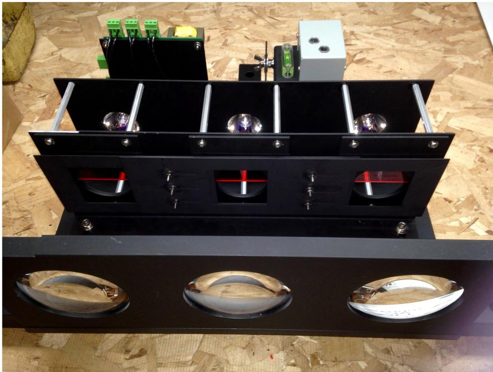
It is most convenient to have the tilt switch function disabled so the unit(s) will not shut down because of unusual elevation angles which may be required during the setting process. This is accomplished by jumpering the tilt terminals in the power and control cabinet of the voltage powered PAPI (see Photo 1) or by jumpering each light unit of a current powered system (see Photo 2).
