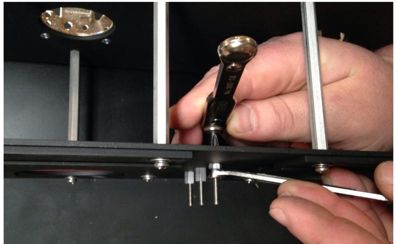
3) Add (1) #6 Washer part # 99-00090 to all screws except the center, left screw (pointed out below).
