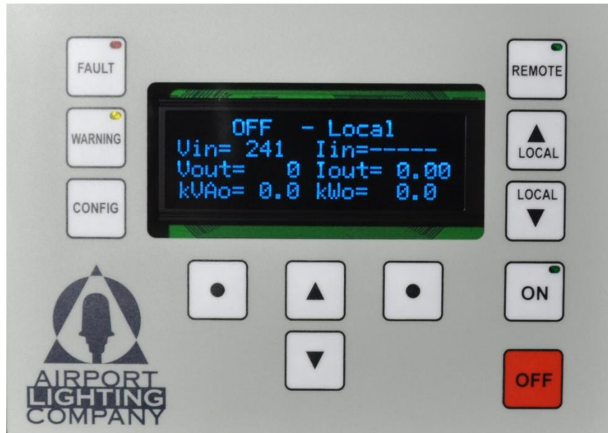
Figure 2: Keypad and Display of a 240V input CCR
