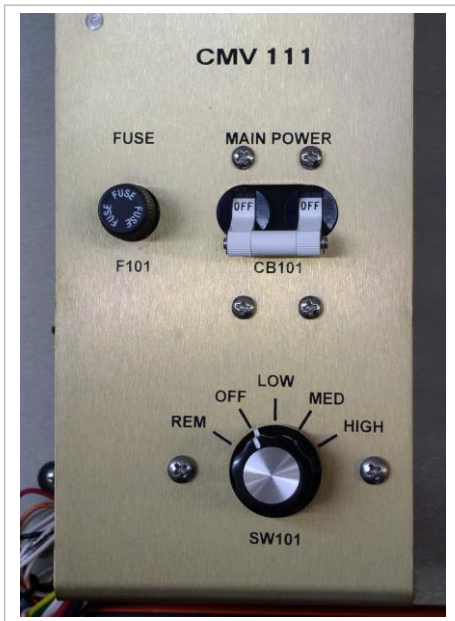
Figure 11a CMV-111 Control Module
